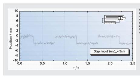
Response of a P-841.10 to a 3 nm peak-to-peak square wave control input signal, measured with servo-control bandwidth set to 240 Hz and 2 msec settling time. Note the crisp response to the square wave control signal.
