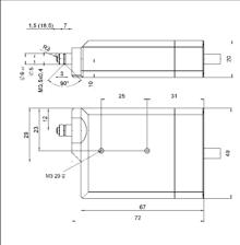
M-232, dimensions (in mm). Cable length: 500 mm, 15-pin sub-D connector with integrated line drivers
